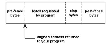
This figure shows the layout of heap debugger overhead in a block. The pre-fence, slop, and post-fence are optional. See "slop=n" on page 7-54.
