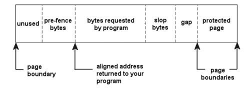
This figure shows the layout of heap debugger overhead in a block with hardware overrun protection. The pre-fence and slop are optional. See "slop=n" on page 7-54. The gap may be zero sized; otherwise it typically is filled with the post-fence fill byte.
