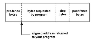
This figure shows the layout of heap debugger overhead in a block. The pre-fence, slop, and post-fence are optional. See "slop=n" on page 7-58.
