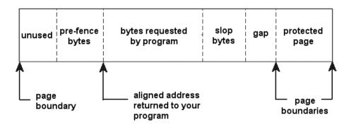
This figure shows the layout of heap debugger overhead in a block with hardware overrun protection. The pre-fence and slop are optional. See "slop=n" on page 7-58. The gap may be zero sized; otherwise it typically is filled with the post-fence fill byte.
