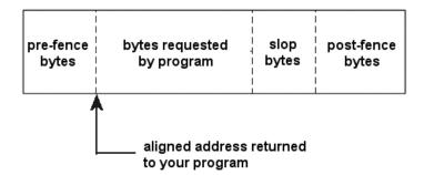
This figure shows the layout of heap debugger overhead in a block. The pre-fence, slop, and post-fence are optional. See "slop=n" on page 6-59.
