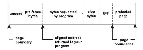
This figure shows the layout of heap debugger overhead in a block with hardware overrun protection. The pre-fence and slop are optional. See "slop=n" on page 6-59. The gap may be zero sized; otherwise it typically is filled with the post-fence fill byte.
