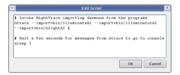
Figure 5-57. Script for Invoking NightTrace in Stream Mode
