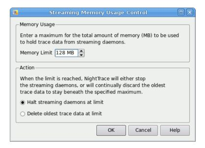
Figure 9-8. Streaming Memory Usage Control Dialog
