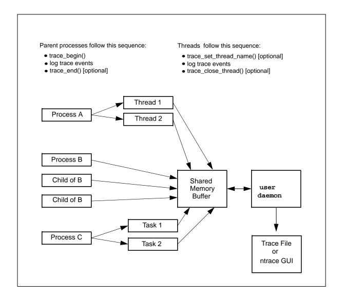
Figure 2-1. Inter-Process Communication and Library Routines
