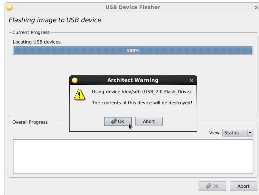
Figure 1-40 Flash Device Confirmation
