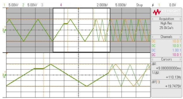
This time, we are demonstrating a smart-seamless transition of two channels. The operation is the same as Seamless Operation but the distance from the end of the flat line (when the clock is restarted) to the point where the two waves change frequency shows approximately 10ms. The smart seamless operation
