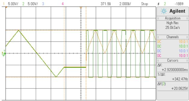
This is the same wave where we zoom into where the transition of the waves occurs. In this case, all waves start at zero offset.
