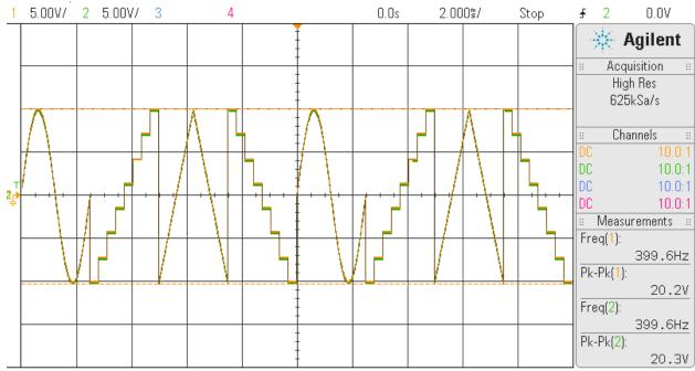
Two waves (Ch0 - yellow & Ch31 - green) displayed above using the wave generation. They were both started at the same time and running at the same frequency of 400 Hz. They are placed one on top of the other to show that they are in phase. During this run, all 32 channels were running the same wave at 400KSPS.
