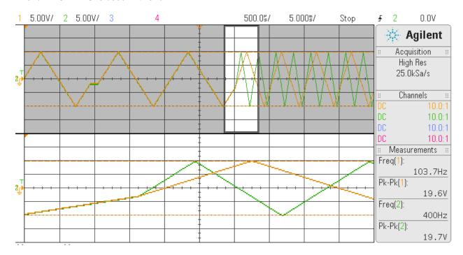
Same wave run as above, however, zooming into the region where the wave change is occurring from 100Hz to 200Hz (Ch0-yellow) and 400Hz (Ch31-green).
