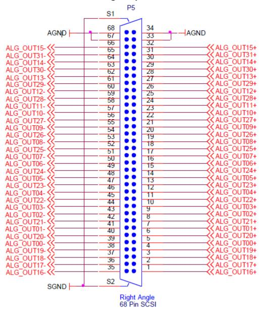
>>>An analog ground connection is always required for the ESD and over/under voltage protection circuits to function correctly.
