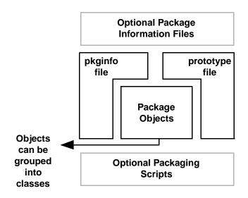
Figure 14-1. The Contents of a Package
