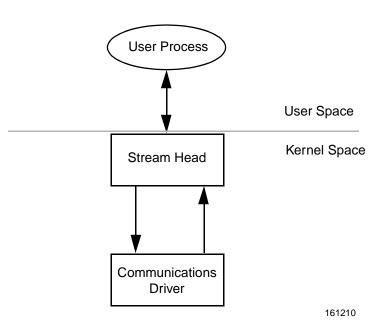
Figure 3-2. Stream to Communication Driver
